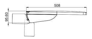
**Type IRIS 2** SCx - 0,029 m<sup>2</sup> The max mounting height - 15 m
